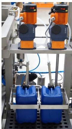
Dosing pump is for LYE or ACID only
