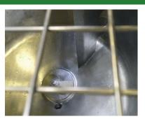
The Sol 3 is specially designed for dissolving powders fast without "fish eyes" or lumps. The powders are added from the top. This mixer is typically used for pre-mixing. Suitable for production where manually cleaning is preferred.
